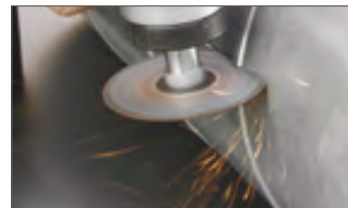
Thin cutting disc ZIP HP: 75x1,0x9,53 A60SX
