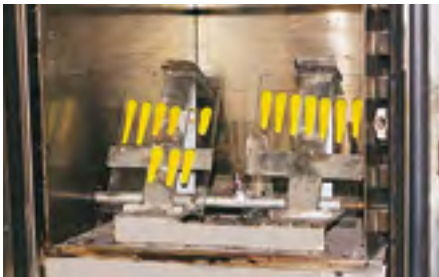
Creep test for phenolic resin powder.
