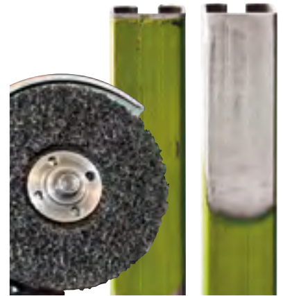
Before and after SCRUBBER pass on a stove enamelled tube.
