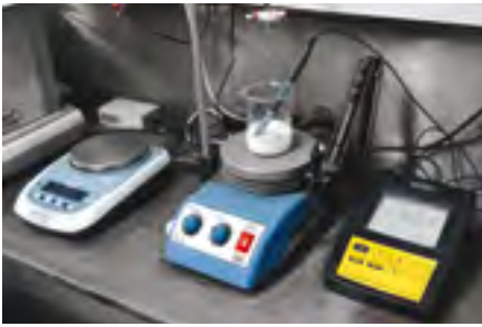
PH metric titration of resin powder.
