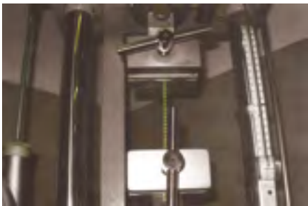
Yarn resistance test of fiberglass reinforcements.
