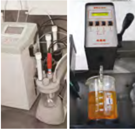
Titration of chemical compounds. Determination of viscosity.
