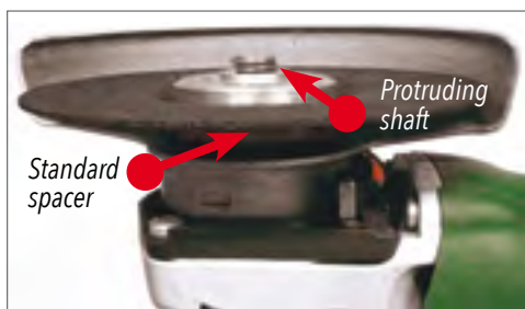
SHAFT PROTRUSION WITH A STANDARD SPACER
